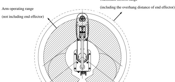
Figure 3-1 Working Range for Robot
