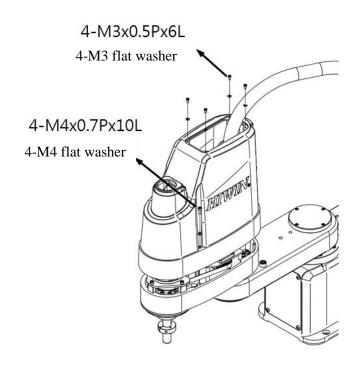
Figure 5-2 Illustration of Dissembling Cover for Robot
