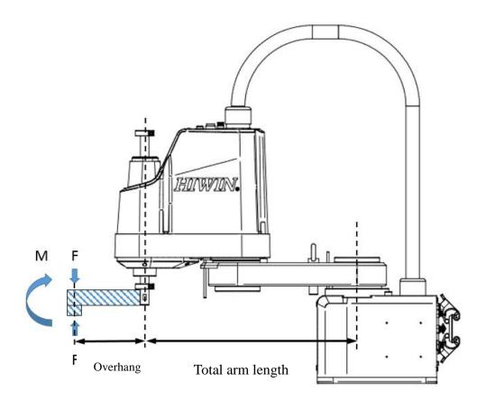
Figure 4-2 Illustration for Calculating Static Torque of Robot End
