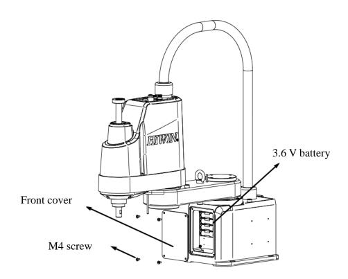
Figure 5-8 Illustration for replace batteries
