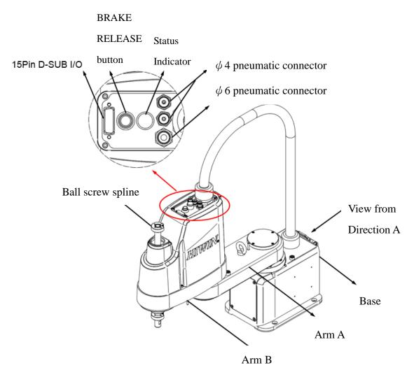
Figure 2-1 Part Names on Robot
