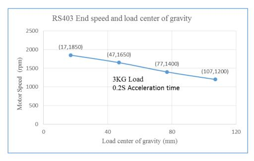
Figure 4-5 \ Load center of gravity and motor speed for 3KG load, spline length 330mm
