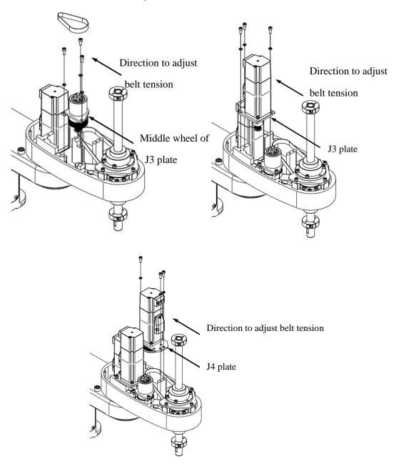
Figure 5-3 Illustrations for Adjusting Belt Tension
