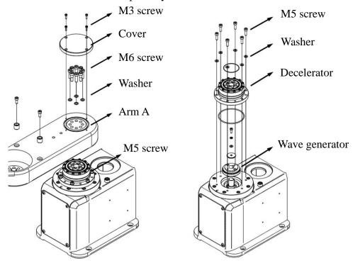
Figure 5-6 Illustrations of Dissembling Decelerator for Robot J1
