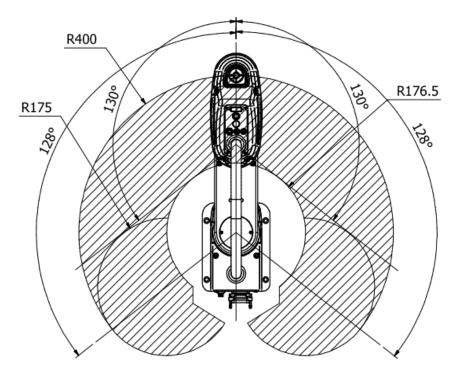
Figure 2-4 Motion Range for Robot
