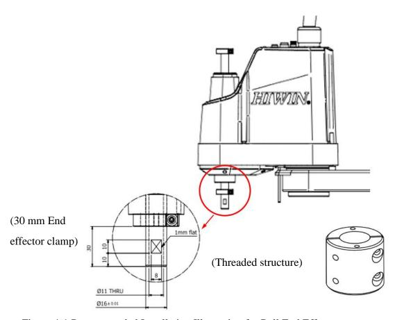
Figure 4-1 Recommended Installation Illustration for Ball End Effector
