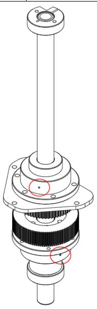
Figure 5-5 Illustration for Lubricating Ball Screw Spline
