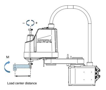
Figure 4-3 \ RS403-400-150-N arm end extension load diagram
