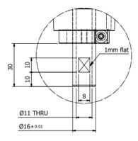
Figure 2-3 Part Dimensions for Robot
