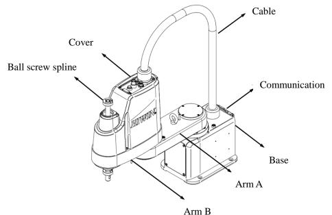
Figure 5-1 Illustration of Part Name for Robot
