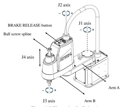
Figure 1-2 Illustration for Robot Axes
