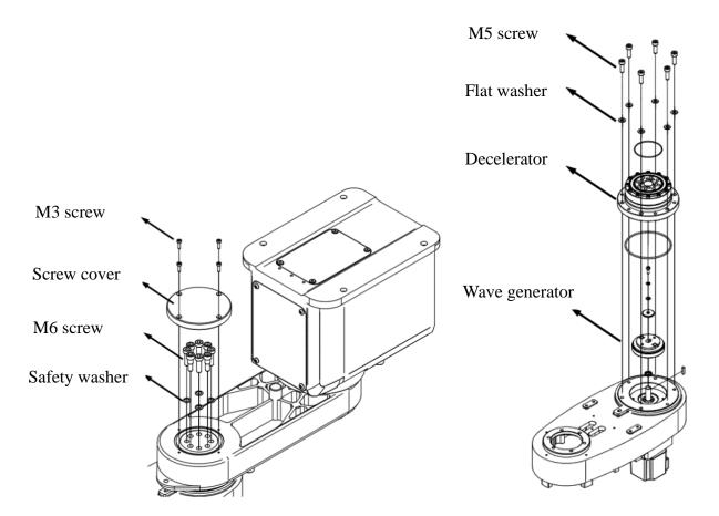
Figure 5-7 Illustrations of Dissembling Decelerator for Robot J2
