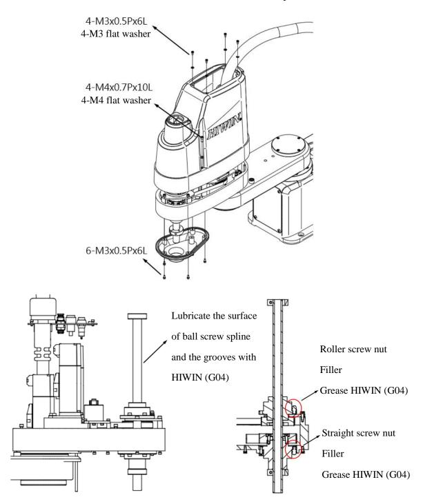
Figure 5-4 Illustration for Lubricating Ball Screw Spline
