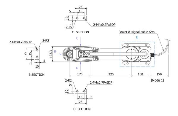
[Note 1] Cable bending radius of at least 150mm, please reserve space to deploy the cable.
