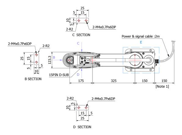
[Note 1] Cable bending radius of at least 150mm, please reserve space to deploy the cable.
