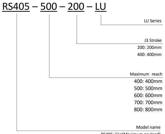
RS405: 5kg(Maximum payload) RS410: 10kg(Maximum payload)
