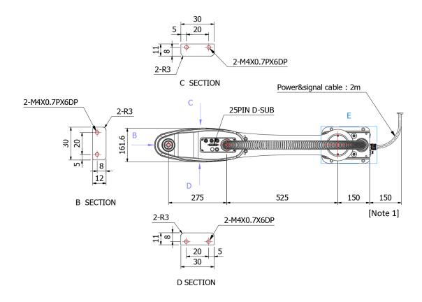
[Note 1] Cable bending radius of at least 150mm, please reserve space to deploy the cable.
