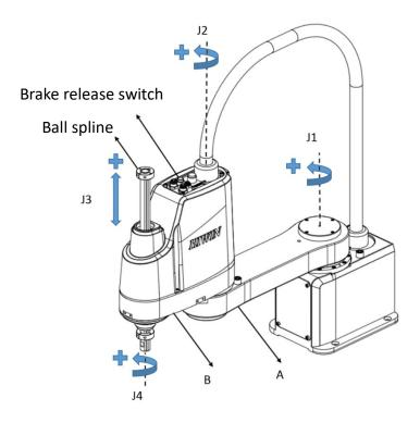
J1 axis: Push the A-arm by hand. J2 axis: Push the B-arm by hand.
